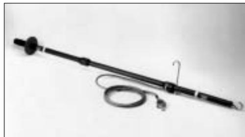
**High-voltage Discharge and Grounding Stick,**
